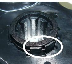
3. Ensure the chainguard is securely snapped on to the crank.
