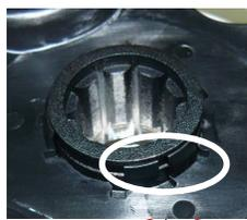
The chainguard is wedged it'self well to the crank see detailed illustration as below.
