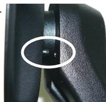
1. Place the chainguard on the crank and ensure the chainguard's alignment pin and crank's alignment hole fit together during assembly.
