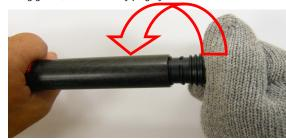
4. Turn the battery plug all the way to seatpost.
