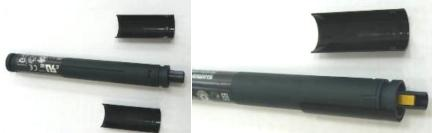
2. Insert the Shimano battery (SM-BTR2) into battery plug.
